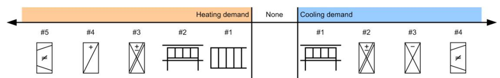
Figure: Sequence of control sequences for a VAV application
